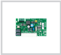
ONE.2WI 433.92 MHz receiver with triple coding: Advanced Rolling Code and Rolling Code, plug-in. 512 memorisable codes.
